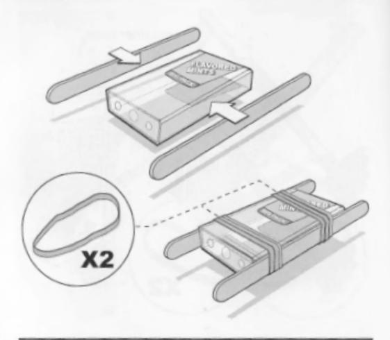
It's time to build the frame out of the Tic Tacs' main container. Fasten two craft sticks to the opposite sides of the container using two rubber bands. The elastic pressure from the two rubber bands may cause some warping at the open end of the container, but minimal warping won't affect the catapult's performance.
