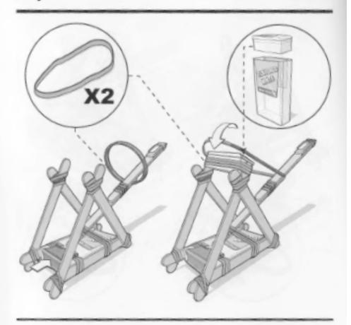
It's time to combine both assemblies. Clamp the arm assembly onto the end of the Tic Tac container frame. Once fastened, the swing arm assembly should move back and forth between the two triangular wooden supports.
