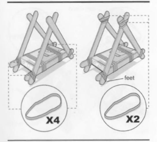
This step requires four craft sticks and six rubber bands. With the foundation of the frame complete, fasten each of the four craft sticks to the endpoints of the container assembly as shown. Once fastened, rotate the sticks to form a triangular frame, then fasten each pair together with one rubber band each. The round ends of these crafts sticks should extend slightly at the bottom to create four feet.
