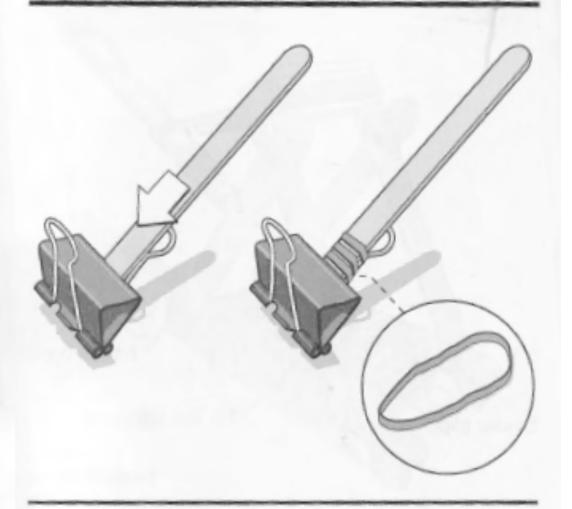
Begin construction with the catapult arm or beam. Locate one medium (32 mm) or similar sized binder clip that can clamp onto a Tic Tic container—test fit it now. Use one rubber band to fasten one craft stick onto the inside of the metal handle attached to the binder clip. Duct tape can be substituted or added for additional strength.
